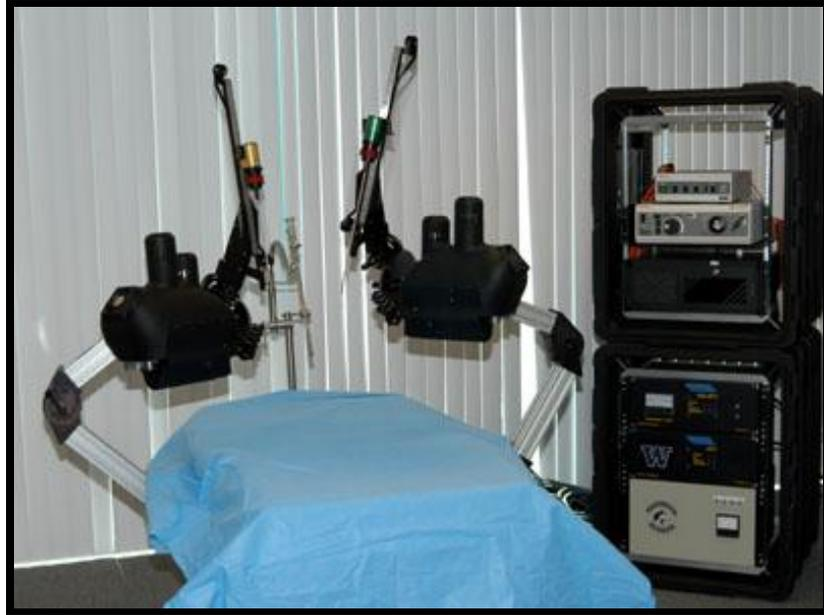
Raven is a surgical robot designed by a research program at the University of Washington in Seattle. Robots are making their way into hospitals around the world. Surgical robots allow precision movements, smaller cuts, faster surgeries, and quicker recoveries.
