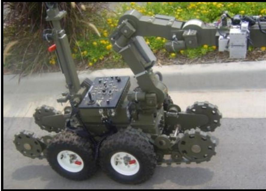
This robot is used by FBI bomb-squads in Oklahoma. It allows access to the bomb without endangering human life as it investigates, moves, and when necessary, disables the bomb.
