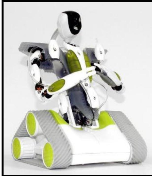
Spykee has built in cameras, microphones and motion detectors, and can send information via WiFi, triggering alarms or alerts on your computer.
