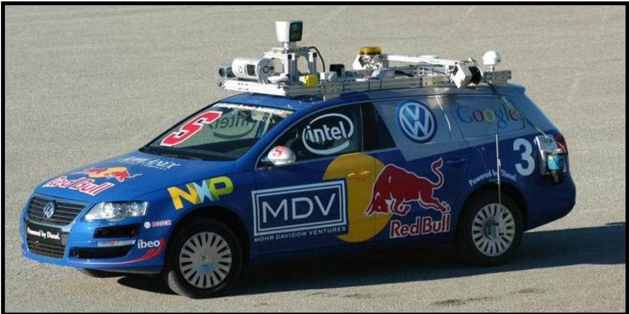
Self-driving cars allow human passengers to set the destination and then sit back while the robotic car makes use of GPS, radar and other information to drive, navigate around other cars, and even parallel park. Shown above is Junior, a Volkswagen Passat whose autonomous programming was developed by the Stanford Racing Team.
