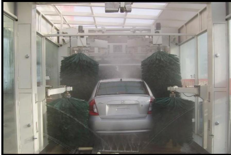
Automatic car washes have taken the labor out of washing your car. Requiring only the push of a button, a moving track brings the car into place while robotic arms equipped with nozzles and brushes take care of the rest.
